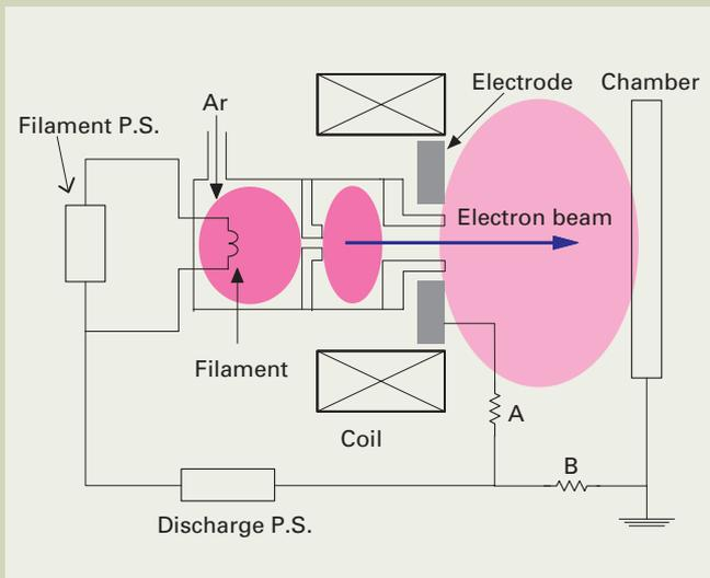
Fig. 2. Schematic diagram of High-Power Built-in Plasma Gun.
