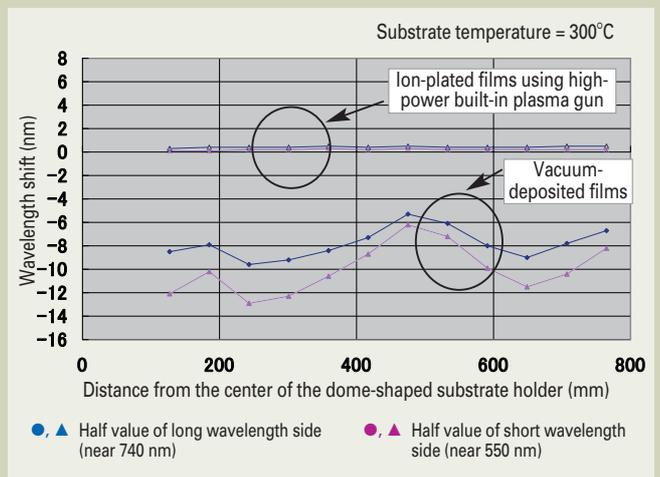
Fig. 5. Wavelength shifts of twelve multi-layer SiO<sub>2</sub>/Ta<sub>2</sub>O<sub>5</sub> films (19 layers).
