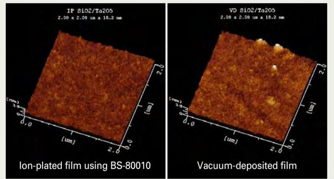
Fig. 7. AFM images of multi-layer  $\text{SiO}_2/\text{Ta}_2\text{O}_5$  Film (19 layers).
